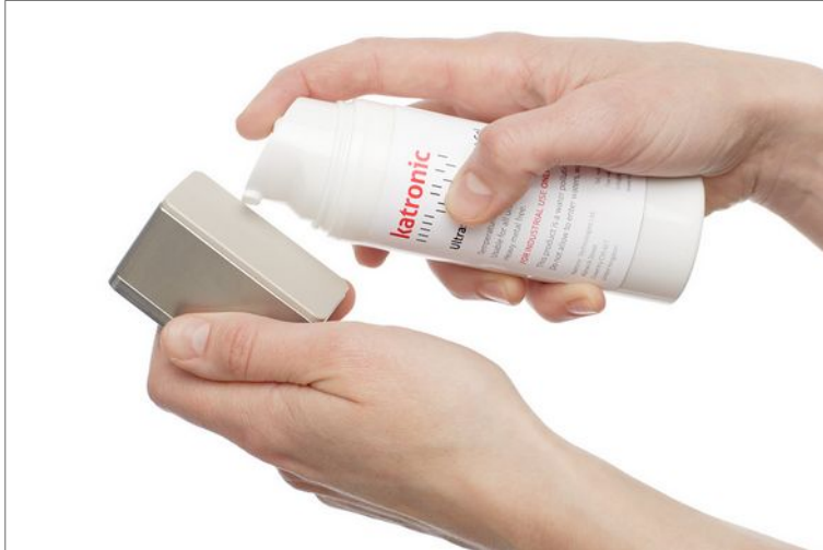
Picture 7: Application of acoustic coupling gel
