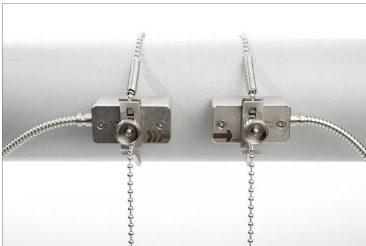
Picture 8: Correct positioning of the sensors
