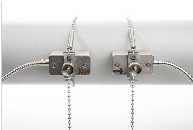
Picture 8: Correct positioning of the sensors
