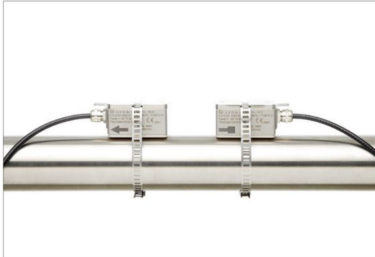
Picture 9: Correct positioning of the sensors
