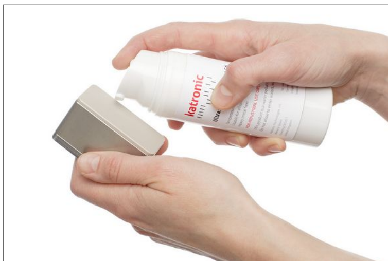
Picture 8: Application of acoustic coupling gel
