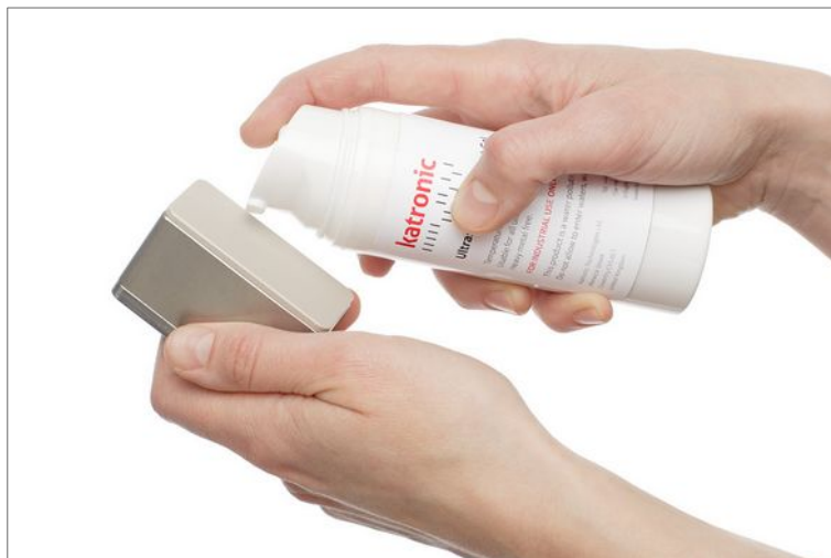
Picture 7: Application of acoustic coupling gel
