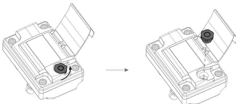
Connect USB cable type mini B. Verify connection by symbol on display
