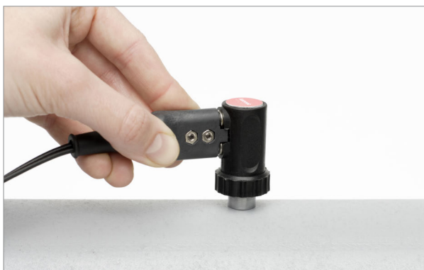
Wall thickness gauge NT in use (alternative design)
