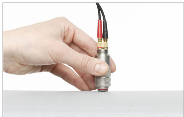
Wall thickness gauge HT in use
