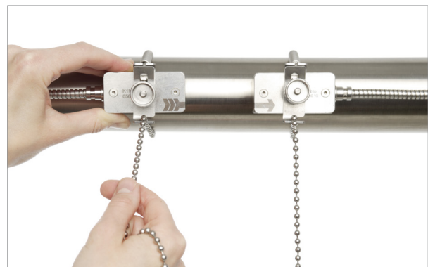
Transducers mounted using chains and clips
