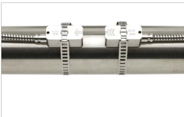
K4N transducers mounted using straps and clamps
