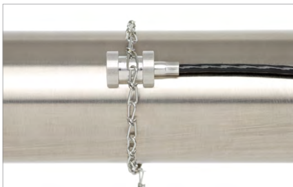
PT100 transducer fixed to pipe
