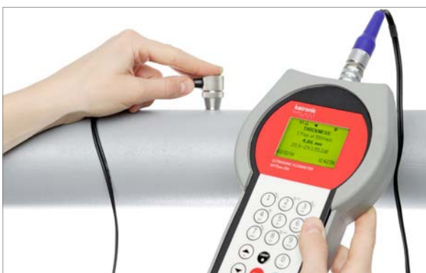
Katronic wall thickness gauge NT with KATflow 200 in use.
