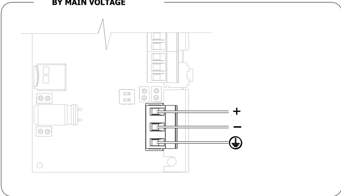
Auto detection of the power source: when main power supply is ON, batteries are excluded and the system operate in continuous sampling mode
