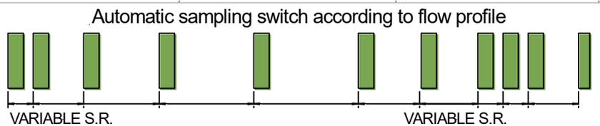
An internal algorithm allows the unit to automatically detect flow rate variations in the process. This capability determines the automatic setting of the sampling frequency. No variations means lower sampling frequency, with less power consumption; high variations means higher frequency to follow the changes in the process.
