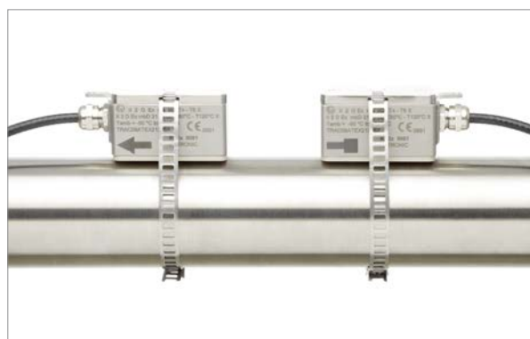
K1Ex transducers mounted using straps and clamps
