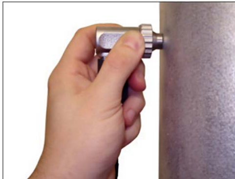
Wall thickness gauge NT in use
