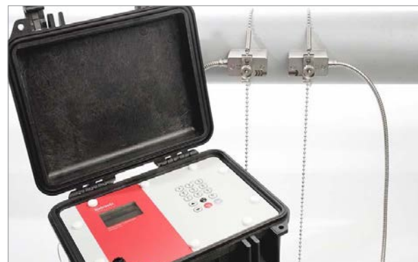
KATflow 210 in operation
