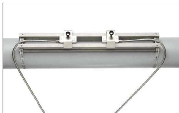
Example mounting rail with transducers
